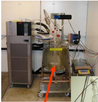
20 litre reactor system
