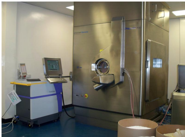
Terahertz sensor mounted directly in pilot scale film coater
