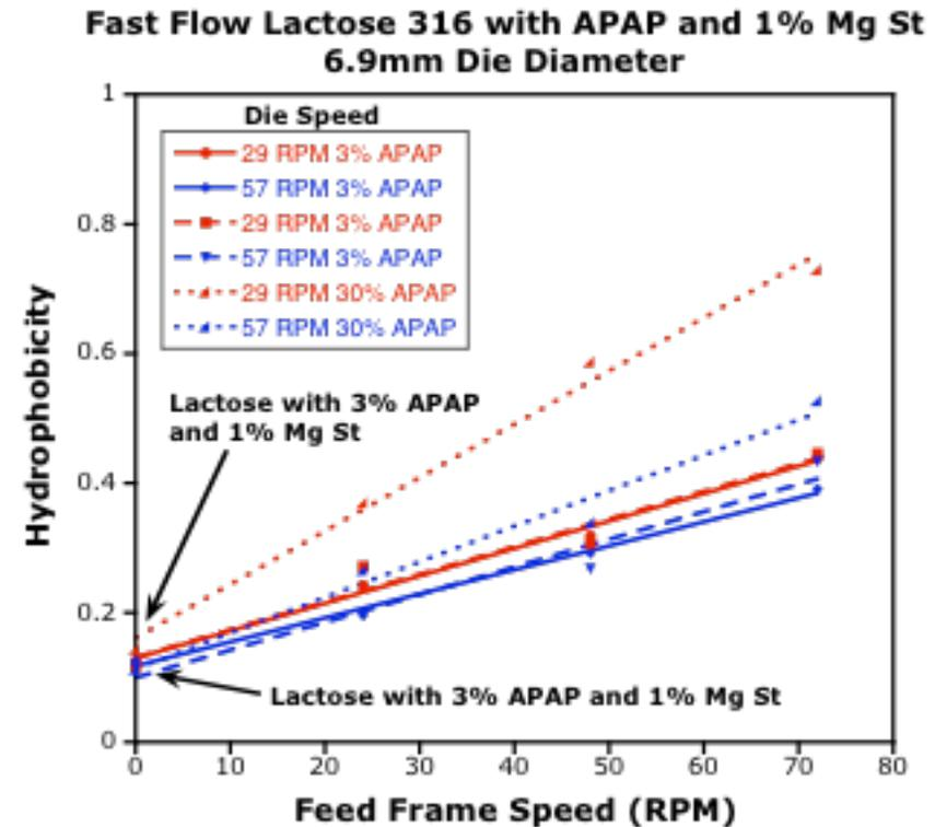
The hydrophobicity increases with the feed frame speed
