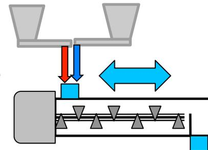
**Radial mixing** required for mixing the initially unmixed powders → Total Shear
