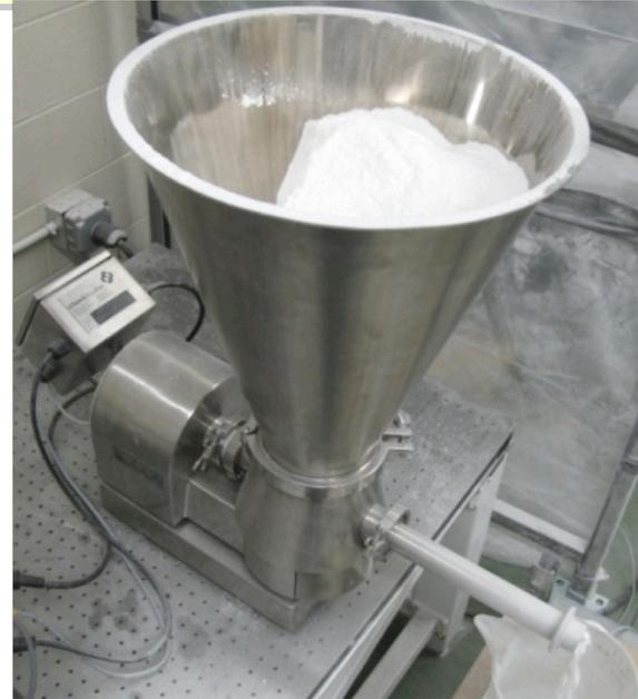
Agitation and hopper flow also affect screw filling consistency.
