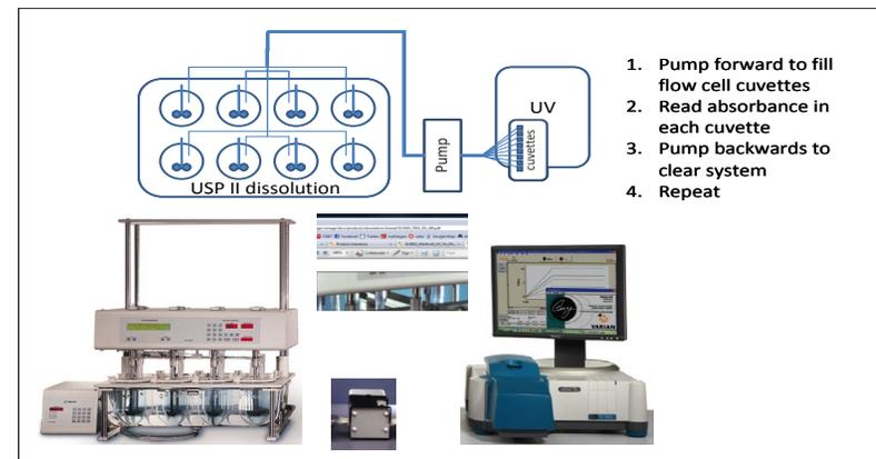
A modified USP method was used for dissolution testing of acetaminophen tablets.
