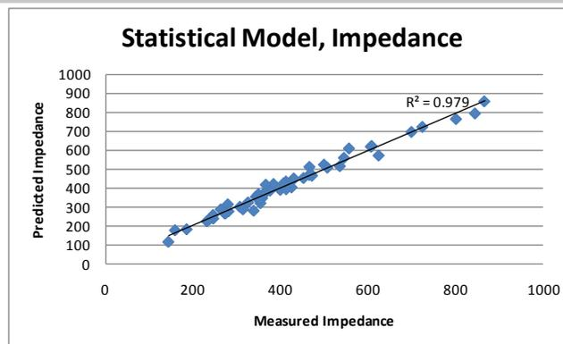
Comparison between predicted and observed values for impedance. The factors blend, shear rate, and strain, and their two-way interactions account for 98% of all the variability in the data set.
