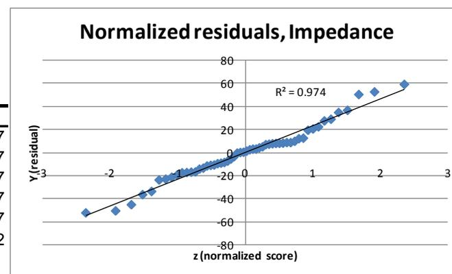
Test of normality for residuals of the observed impedance measurements. The residuals are normally distributed, displaying a  $R^2$  of .97 when compared to a normal distribution.
