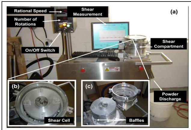
Formulations prepared were sheared at shear rate of 80 rpm and shear strain of 40 rev, 160 rev and 640 rev.
