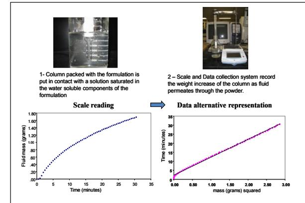
Hydrophobicity was measured from the slope of the squared mass versus time.
