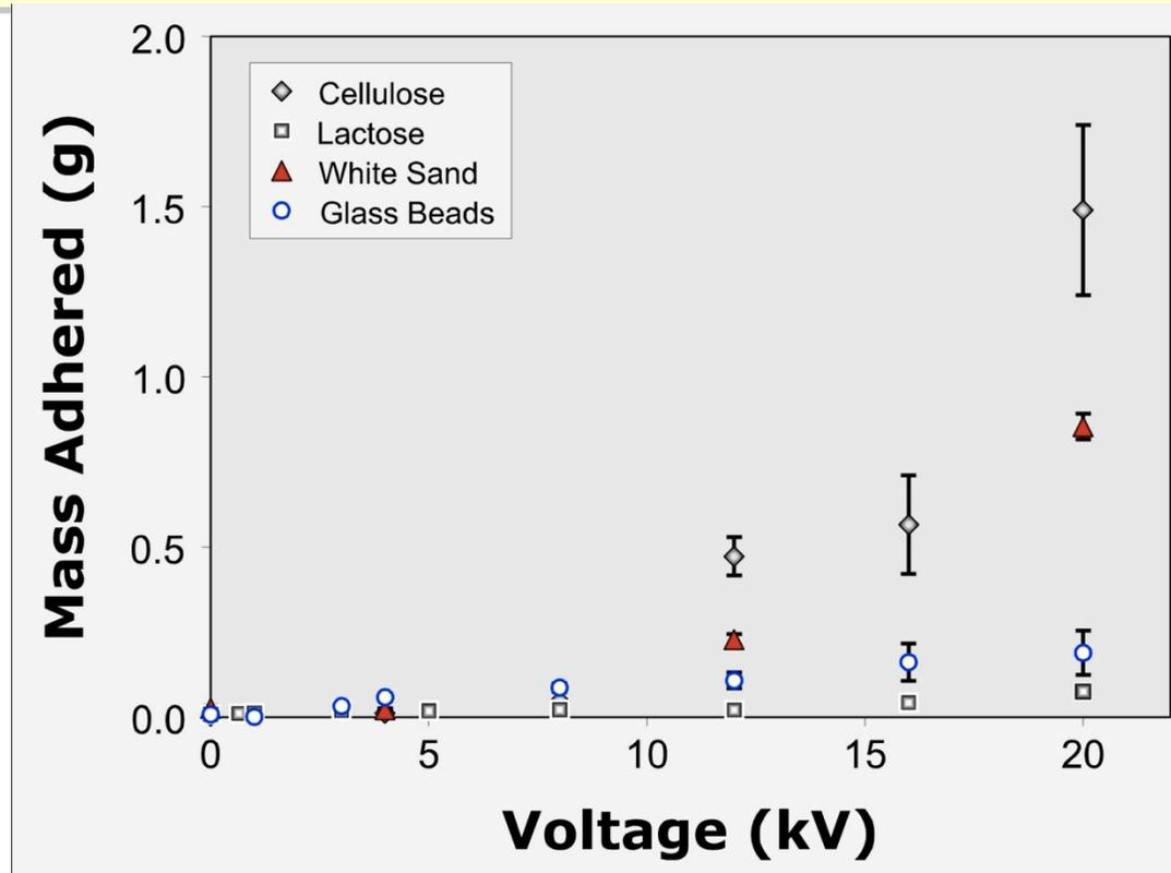
*The mass of material adhered to a grounded rod as a function of the voltage of the VDG. As the voltage increases so does the strength of the electric field allowing more material to adhere to the rod.*
