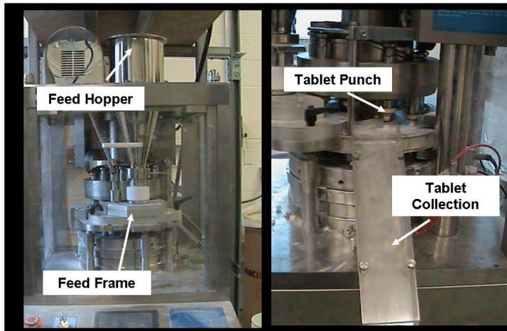
Powders were compressed into tablets at a compression force of 12 kN.
