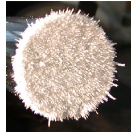
Cellulose adhered to a charged rod
