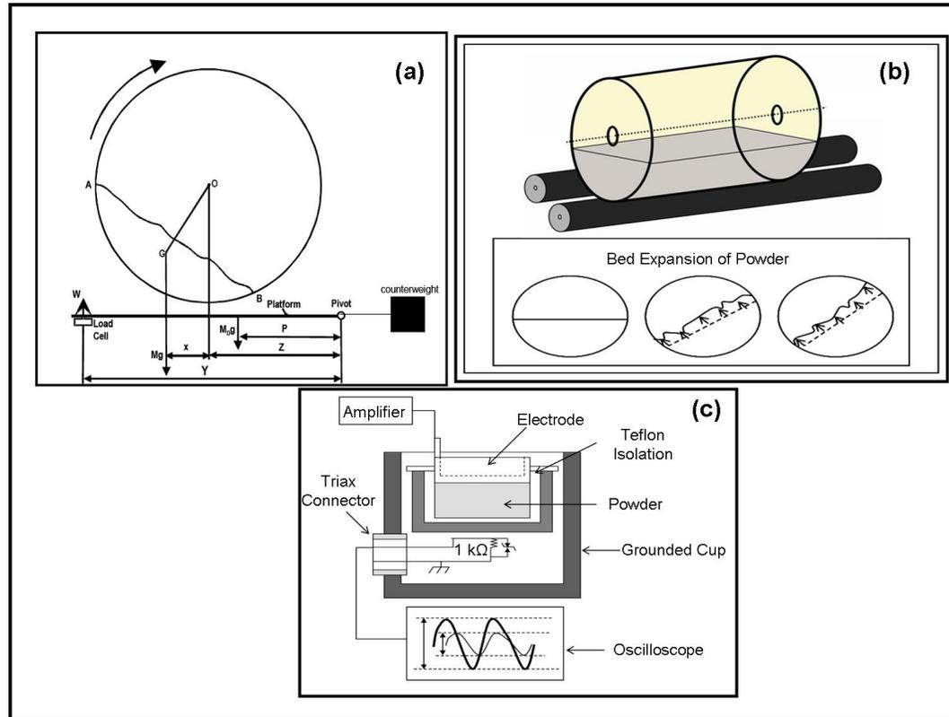
Laboratory equipment for the measurement of flow and electrical properties of pharmaceutical powders (a) Gravitational Displacement Rheometer (GDR) to measure flow index (Alexander et al., 2006) (b) Dilation rollers with cylinder filled to 40% powder for measuring bed expansion (c) Impedance measurement using oscilloscope, faraday cup and amplifier.
