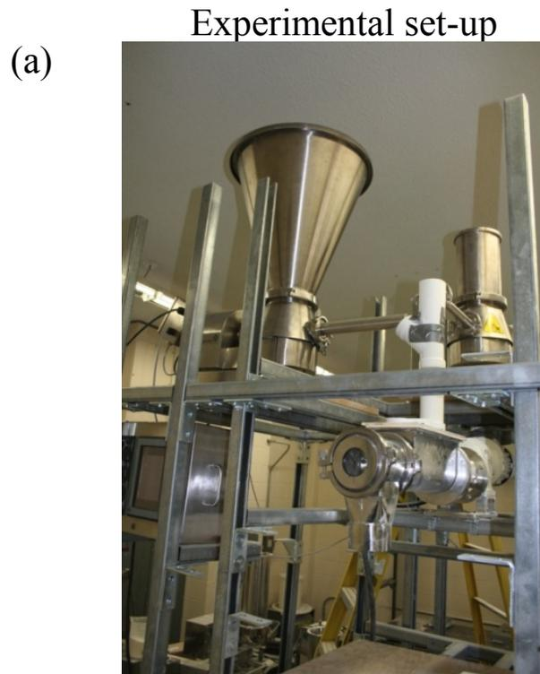
Gericke continuous mixer integrated with Schenck AccuRate LIW feeders
