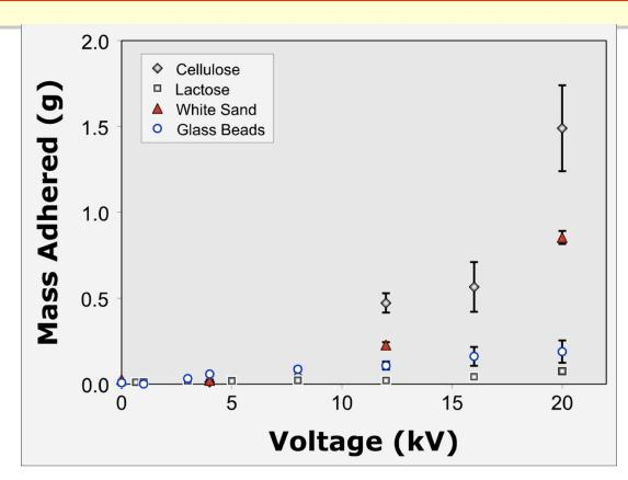
The mass of material adhered to a grounded rod as a function of the voltage of the VDG. As the voltage increases so does the strength of the electric field allowing more material to adhere to the rod.
