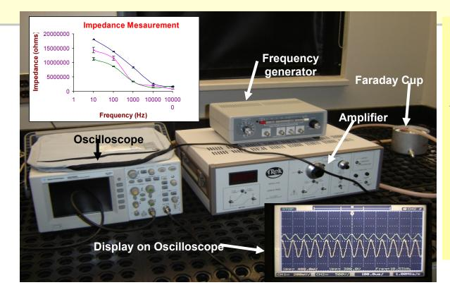
The Model 610E high voltage (HV) supply amplifier controller supplied by Trek Inc was used for voltage supply.
