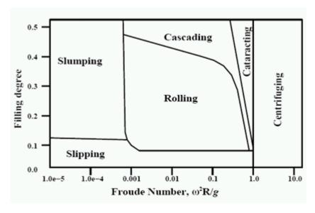
Mixing and segregation in rotating horizontal drums (Metcalfe et al., 1995; Ottino and Khakar, 1995)
