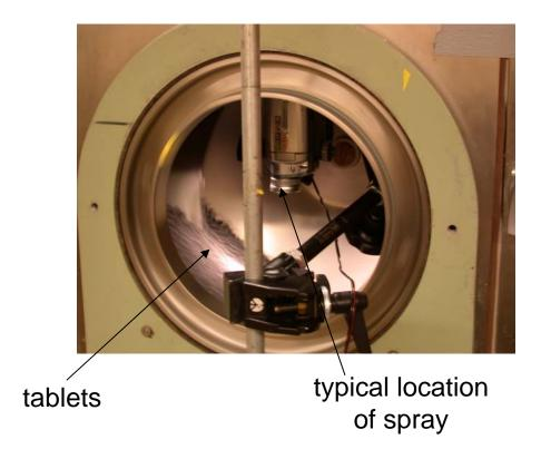
Experiments use ~7 kg load (~15% fill level in drum) of biconvex tablets
